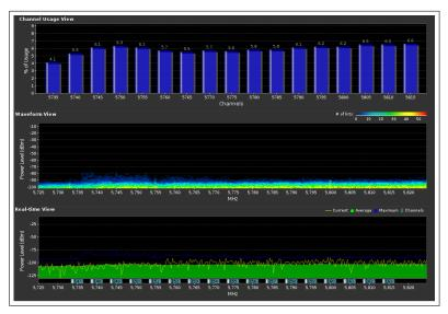
To the east of St. Mary's 75MHz is usable, with a noise floor below 90dBi. This is enough spectrum for three or four high throughput point-to-point links:
