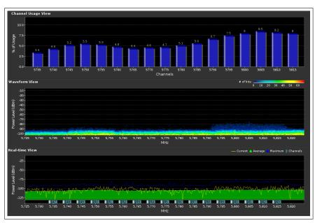
To the south of St. Mary's there is 65MHz of clean, usable spectrum, which should be more than enough to build the requisite links:
