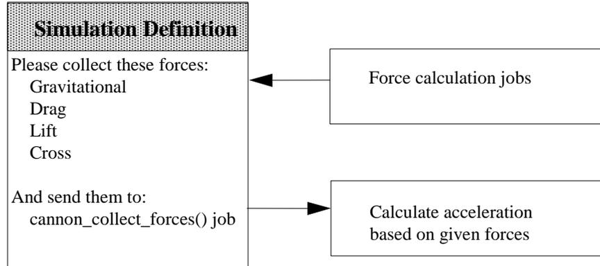
Figure 71 Simulation Definition With Collect Statement – S\_define
