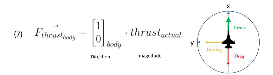
So, the magnitude of the thrust force vector is thrust<sub>actual</sub>, and the direction is [1,0] in Body coordinates.
