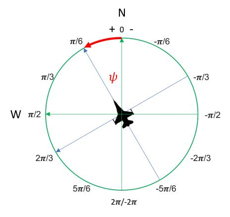
If the aircraft is moving directly north,  $\psi = 0$ . Directly west is  $\pi/2$ . Directly east is  $-\pi/2$ .
