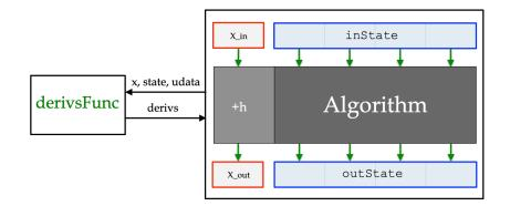
Derived classes should override this method to calculate outState using some integration algorithm, using X\_in, inState, and derivs\_func, and default\_h. The over-riding method should also pass the user\_data when calling the DerivsFunc. The default algorithm is Euler.
