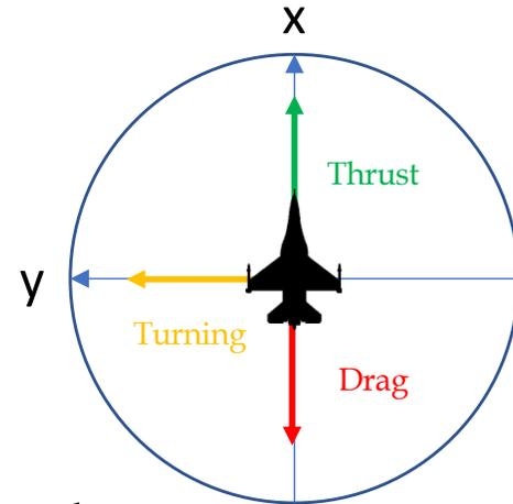
Like our desired speed, just we want something doesn't mean that the aircraft is capable of it. In our case we need to limit the magnitude of our force to 1 G ( force of gravity), that is  $9.8 \text{ m/s}^2 * m$ . So if our mass is 5000 kg, we need to limit our turning force to between -49000 .. 49000 Newtons.
